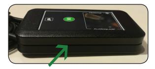
A few mm behind this hole there are two pins. When the user makes an electrical connection between these two pins (e.g. with a paperclip) the Optima6 emits a short beep, and restarts.
